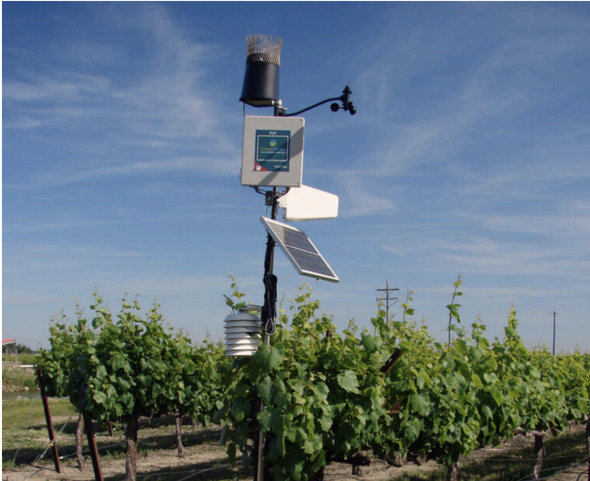
Fig. 2. Monitoring atmospheric conditions and soil moisture within a vineyard using a weather station. LODI Wine Growers.
